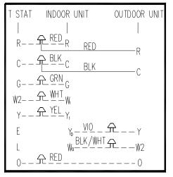
Fig. 3 - Heat Pump Application wiring.
