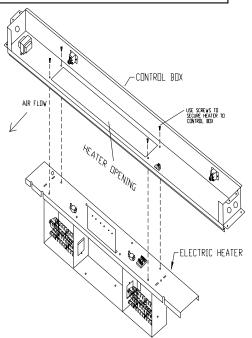
Fig. 1 - Heater assembly
