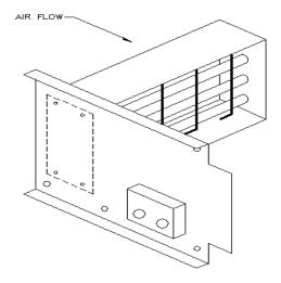
4. Connect power wiring as shown in schematic diagram. All connections should be made inside the package unit and comply with National Electric Codes, State and Local Codes. Heaters with factory installed fuses or circuit breakers may be installed on a branch circuit protected by either a fuse or a circuit breaker. For all other heaters, the branch circuit must be protected by a fuse or a circuit breaker supplied by others.
