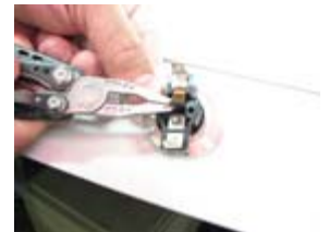
A photo of a typical automatic reset thermostat, used as an over-temperature limit, showing contacts that were welded together as a result of excessive cycling.
